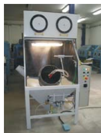
Injecting blasting cabin of TM 1000 type with rotating drum
