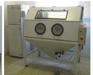
Injecting blasting cabin of TM 1500 type with suction filter
