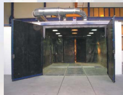
The blasting area 8 x 5,5 x 3,5 m passable with whole-surface automatic collection of abrasive and floor covered with porous grates
