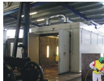
Blasting area 8 x 5 x 4 m with periphery walls and ceiling from sandwich panels supplied with compressor plant of similar design
