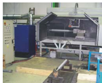
Injecting blasting cabin with double-bent doors for blasting of cylindrical parts before application of plasma coating
