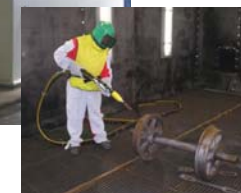
Blasting area 8 x 5 x 4 m with periphery walls and ceiling from sandwich panels supplied with compressor plant of similar design
