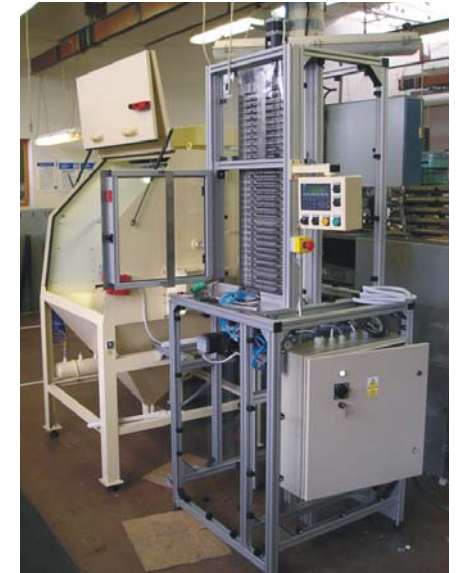
Special blasting cabin for electro-technical industry
