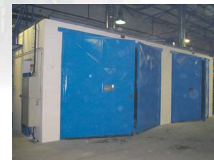
Two blasting areas each for different type of abrasive (inner sizes 6 x 5 x 3,5 m and 6 x 4 x 3,5 m)
