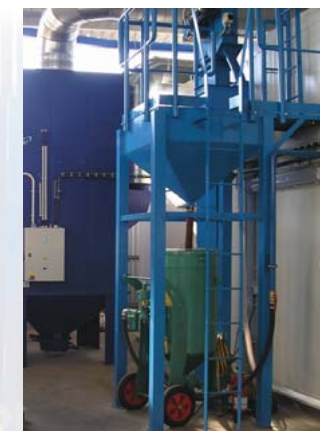
Technological fitting of blasting area composed from bucket conveyor, rotating sorter, abrasive storage, pressure boiler, and suction filter
