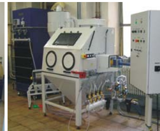
Special blasting cabin for blasting of pressure parts from plastics by plastic abrasive
