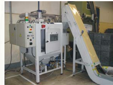
Special blasting equipment for blasting of bearing rings
