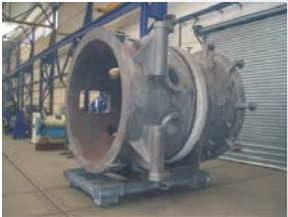
Fusion section of cupola furnace
